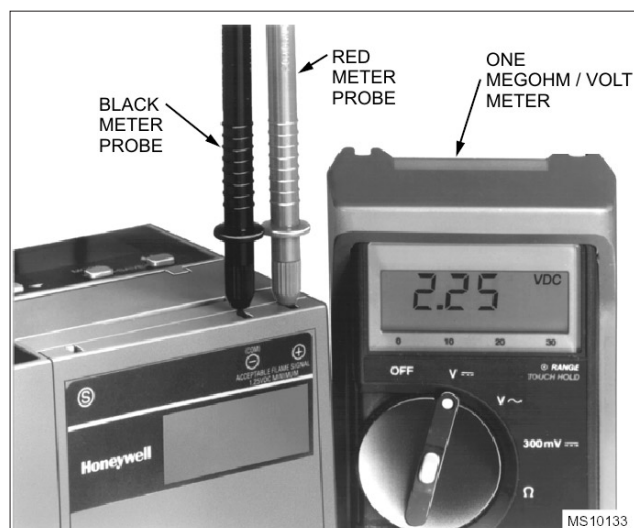
Fig. 11. Measuring voltage flame Signal with 7800 SERIES controls
